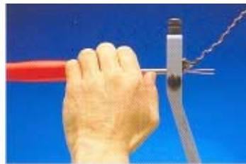
6. For the larger cable sizes or as an alternative to the MIC Stripper the ZSU stripping tool can be used.
