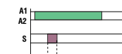
Delay off after closing and opening of external contact and relay energising (e)
