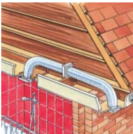
A typical shower room installation
