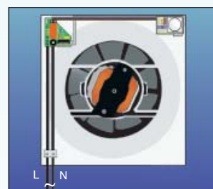
Mini T and Sensor, easy timer adjustment by small control knob.
