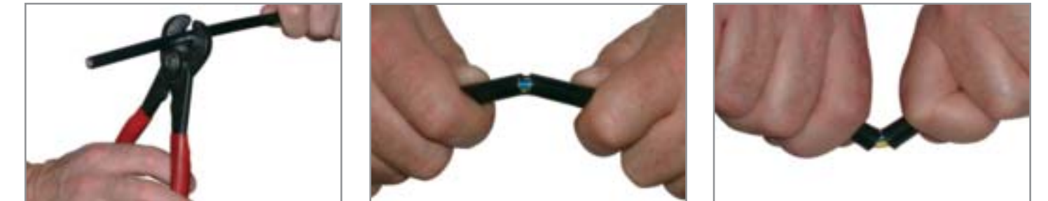
Ring the cable to slice through insulating sheath.
